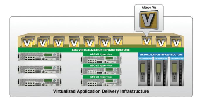
Radware's Alteon Virtual Appliance (VA™) is a fully-functional ADC solution packaged as a virtual appliance running on server virtualization infrastructure. It provides identical functionality to Alteon physical ADC devices including local and global server load balancing, Layer 7 capabilities and application acceleration.
